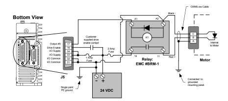
Figure 16: Epsilon Brake Wiring Diagram using the Command Connector
